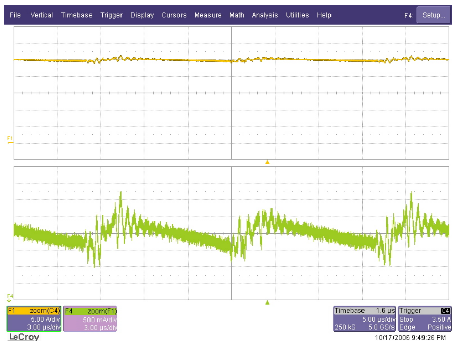
Figure 6.19 Load current waveform (top) and its vertically zoomed version (bottom) at 25% load (scales: 5 A/div, 500 mA/div, 3 \mu s/div).
