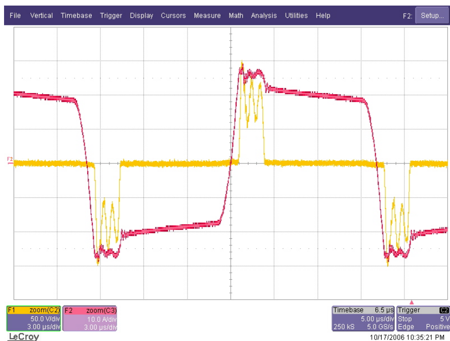
Figure 6.18 Transformer secondary voltage (yellow) and secondary current (red) waveforms at 25% load (scales: 50 V/div, 10 A/div, 3 \mu s/div).
