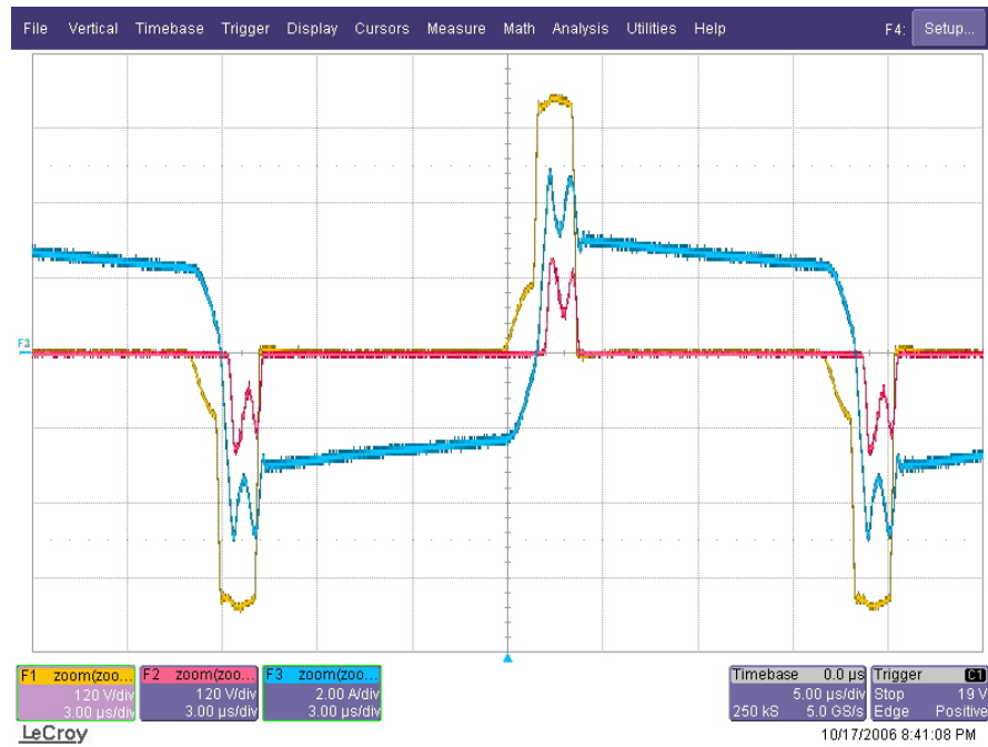
Figure 6.23 Inverter output voltage (yellow), transformer primary current (blue), and transformer secondary voltage (red) waveforms at 15% load (scales: 120 V/div, 2 A/div, 120 V/div, 3 μs/div).
