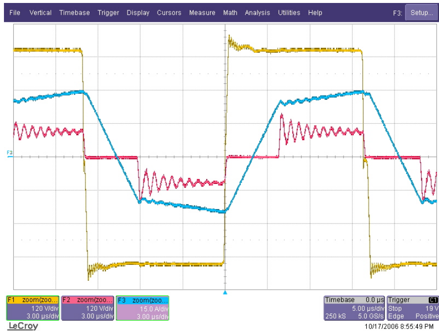
Figure 6.6 Inverter output voltage (yellow), transformer primary current (blue), and transformer secondary voltage (red) waveforms at the rated load current (scales: 120 V/div, 15 A/div, 120 V/div, 3 \mu s/div).
