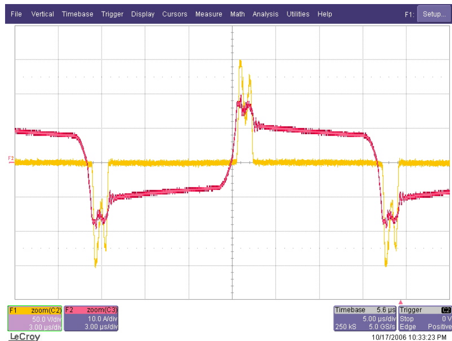
Figure 6.24 Transformer secondary voltage (yellow) and secondary current (red) waveforms at 15% load (scales: 50 V/div, 10 A/div, 3 μs/div).
