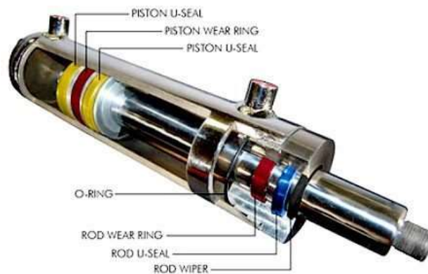
Figure 1.7: Section detail of a hydraulic cylinder [11].
