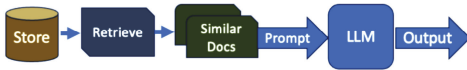
Figure 2.9. Work principle of retriever (Source: Topsakal and Akinci 2023)
