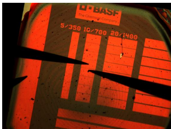
Figure 2-5. Picture of a bottom gate bottom contact OFET covered with a polymer.
