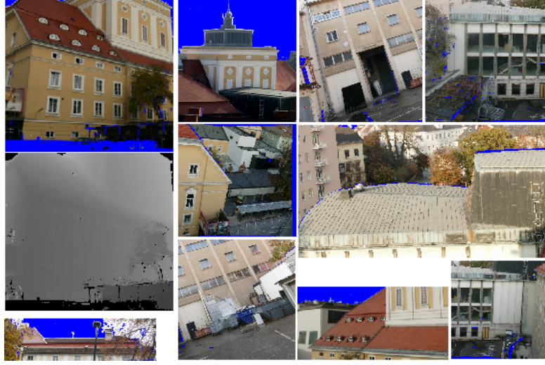
Figure 5.2: 10 of the 20 3D data sets used in the analysis. The points without range information are marked in blue. The gray image shows the range data of the top-left scene. The resolution range is [512-2048]x[390-2290] with an average resolution of 1140x1001.
