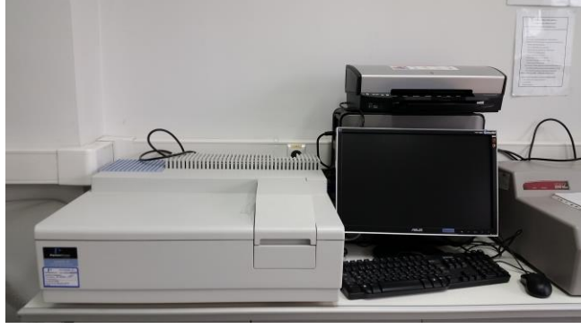
Şekil 5. 9 Perkin Elmer Lambda 35 UV/Vis Systems Spectrophotometer
