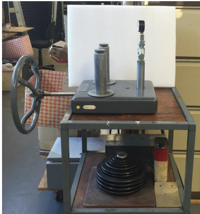
Figure 3.17 Photograph of the deadweight tester.
