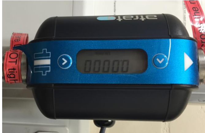
Fig 3.7 Photograph of the flowmeter (Atrato ® ).
