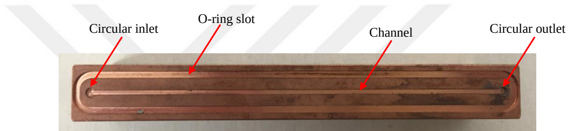
Figure 3.10 Photograph of the test section 4.
