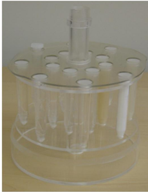
Figure 12 : Test tube phantom holder with 16 test tubes
