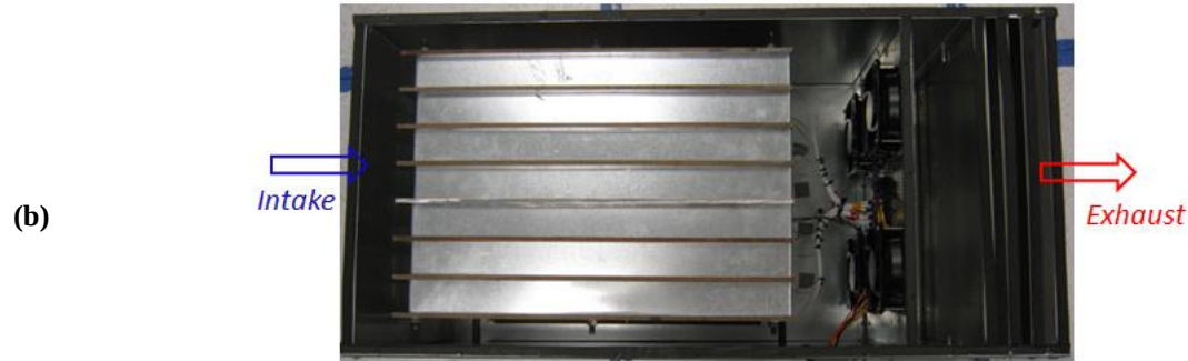
Figure 2.8: Chassis layout: (a) Drawing (dimensions in inch); (b) Photograph from the top (cover removed).
