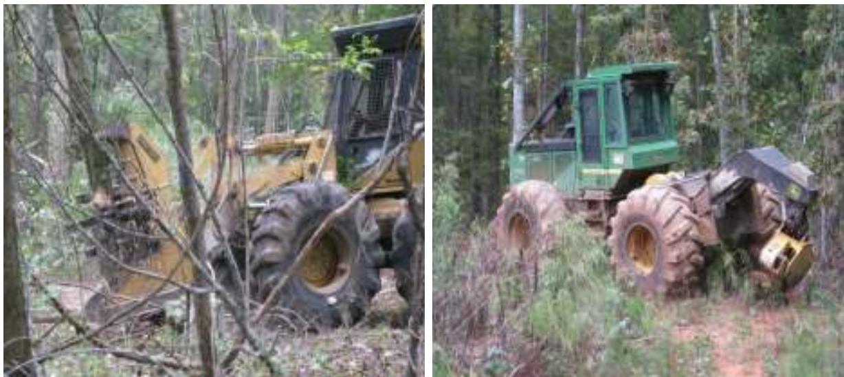
Figure 3.12: Rubber-tired Hydro-AX 411EX model Feller Buncher and John Deere 540 GIII Model Skidder
