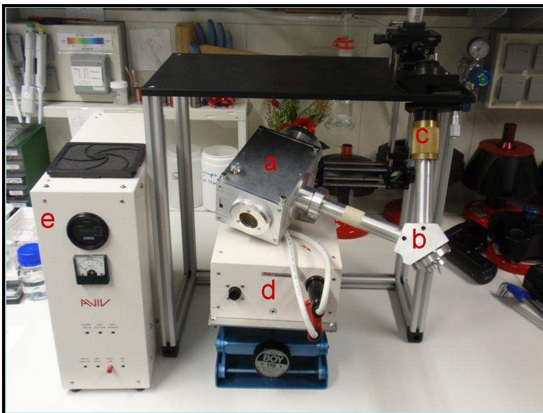
Figure 4-6: Prototype Constant Light Source from Aviv Biomedical
