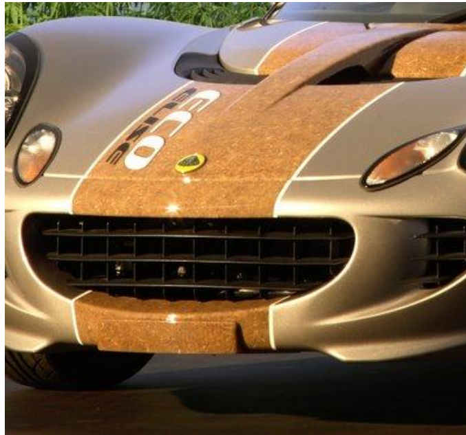
Figure 2.6 A car body (Lotus eco) produced with plant fibre composites ( www.lotuscars.com , 2012).
