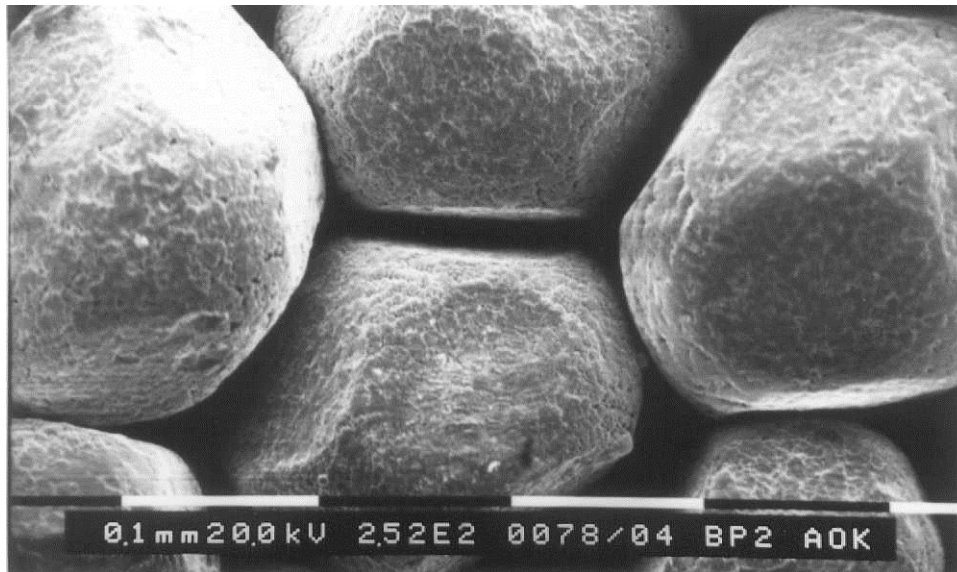
Figure 4.6.7 : SEM micrograph of surface characteristics of bronze powder (220 \mu\text{m} ) compacted at 800 MPa, 250x.
