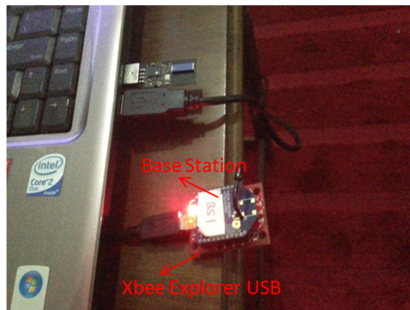
Figure 3.12. Base station connected to central computer.
