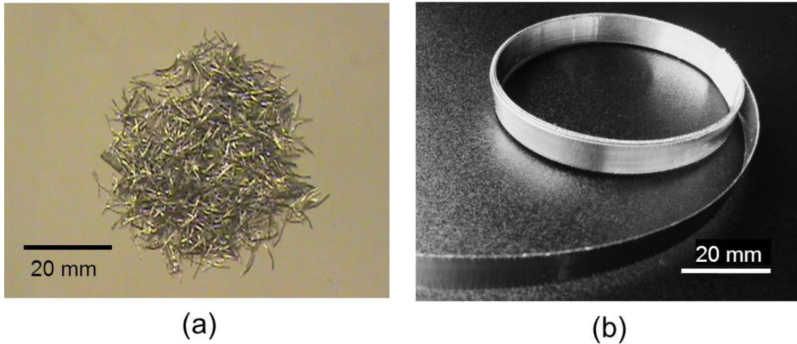
Figure 6-1 MgAZ31B processed by EM: a) LP EM ( V_o = 0.2 m/s, p/2k = 1.1 , T = 70 °C) resulting in discrete needle-like chips and b) HP EM ( V_o = 1.2 m/s, p/2k = 1.7 , T = 230 °C) with chip formed as long continuous sheet. \gamma \sim 2 , T_0 = 25 °C (no pre-heating), t_0 = 0.25 mm (after [11], used with permission of Elsevier).
