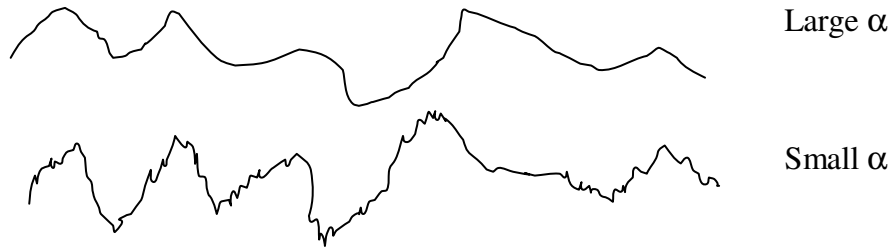
Figure 2.3: Illustration of large and small roughness exponents, \alpha .
