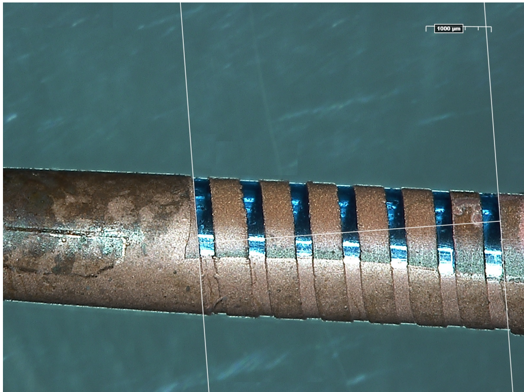
Figure 6.1. LC resonator structure fabricated on 5 Fr catheter.
