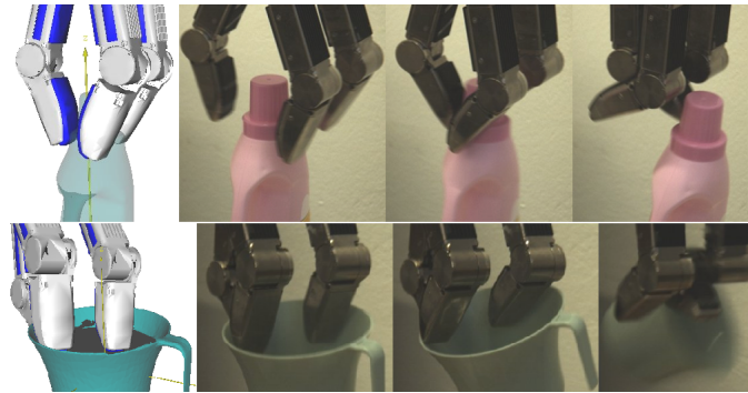
Figure 3.11: Examples of stable grasp hypotheses that failed in the real experiments.
