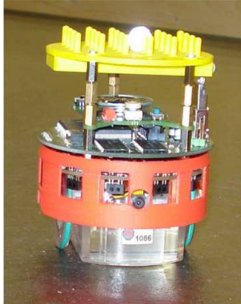
Figure 3.1: An e-puck with Linux board fitted in between the e-puck motherboard (lower) and the e-puck speaker board(upper). Note both the red skirt, and the yellow hat that provides a matrix of pins for the reflective spheres which allow the tracking system to identify and track each robot.
