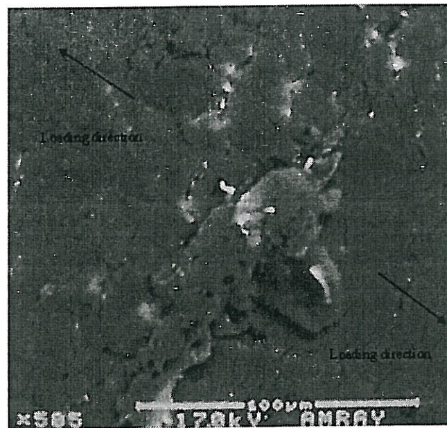
Figure 9.2.3: SEM Micrograph of a Craze Emanating from a Rubber Particle in HIPS.
