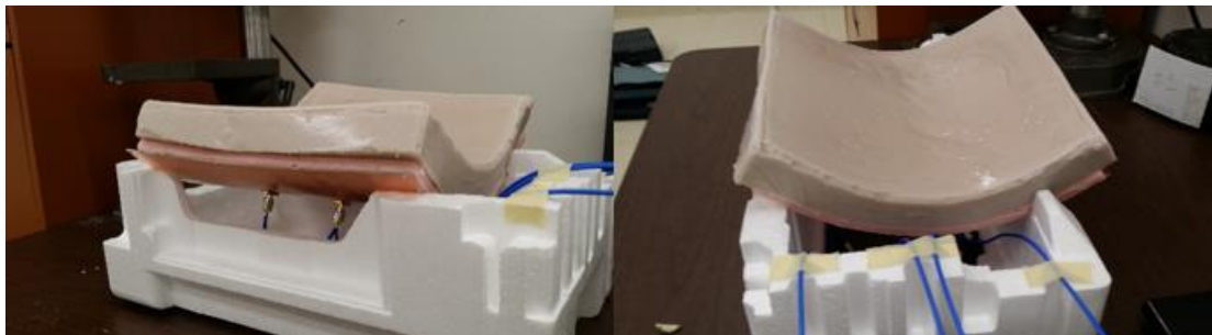
Figure 3.88 Skin and fat layers on the mild HT applicator
