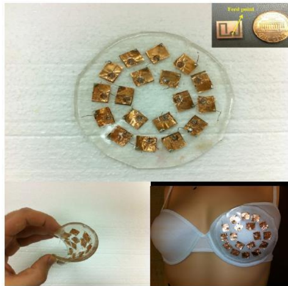
Figure 1.17 Microwave antenna applicator printed on a flexible material (PDMS)
