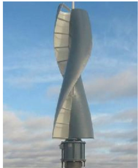
Figure 13 Savonius VAWTs (URL 3) also known as Drag type VAWTs
