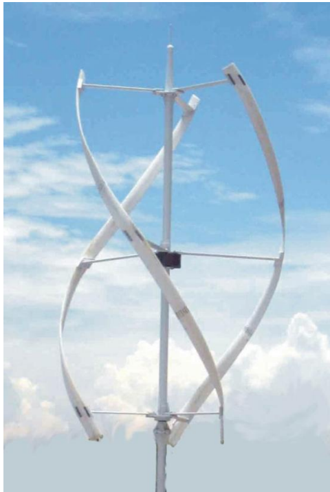
Figure 12 Darrieus VAWTs (URL 2) also known as lift VAWTs
