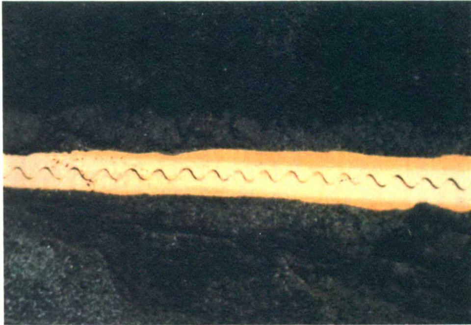
Figure 1.2 Rapid crack propagation in a full-scale test; BP 002-40 250 mm SDR 11 pipe at 0°C. Note sinusoidal weaving of the crack path.
