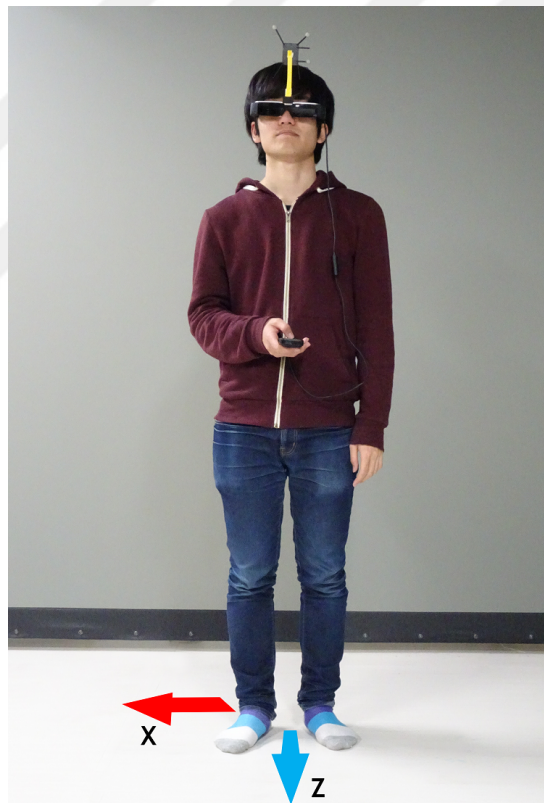
Fig. 4.4: A participant using an HMD with markers for optical 3D motion tracking, having a controller for selection in his hand. Here, he is performing the task with a ray-based technique using IMU.
