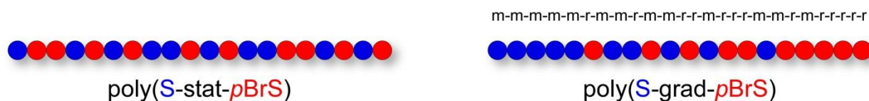
Figure 2.2 Illustrations of the statistical (stat) and gradient (grad) S/p-BrS copolymer sequences synthesized and investigated by Kerr effect measurements. Correlated comonomer and stereosequence gradients in poly(S-grad- p-BrS ) are also shown.
