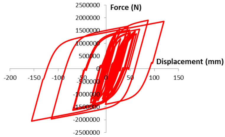
Figure 3.3. Force displacement relationship of temperature dependent material model
