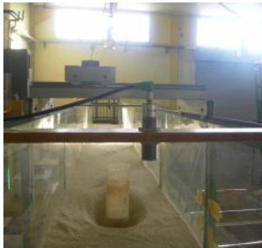
Figure 3.9 Ultrasonic Level Sensor ULS
