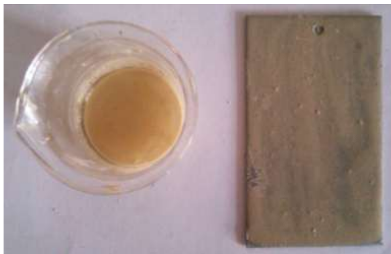
Figure 2.9 Antifouling paint coated metal plate.
