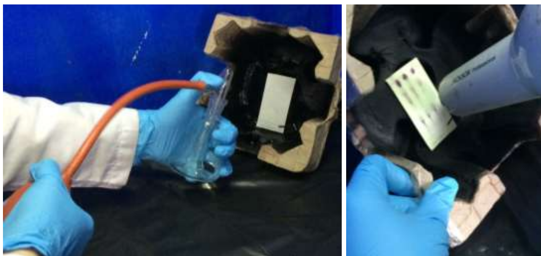
Figure 2.5 Application of vanillin-sulfuric acid on TLC.
