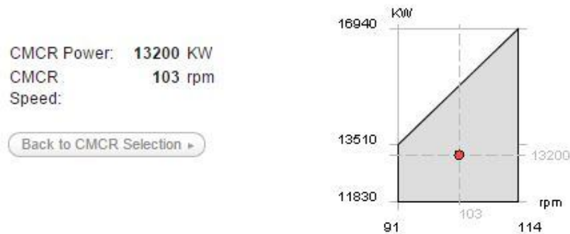
Figure 2. 19: Wärtsilä 7 cylinders engine layout diagram with the contract point (7RT-flex60C-B).
