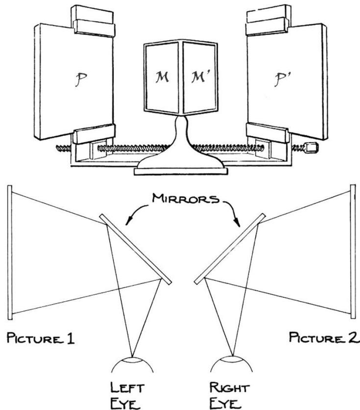
**Figure 2.11:** Wheatstone's stereoscope and its construction (Url-12)
