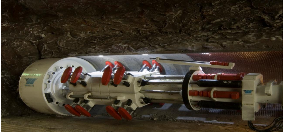
Şekil 2.4: Şiltsiz TBM (Sert Zemin Tünel Açma Makinesi) ( https://www.herrenknecht.com/en/products/core-products/tunnelling/single-shield-tbm.html ).
