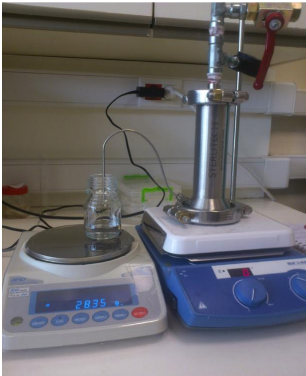
Figure 3.5 : The laboratory-scale of dead-end membrane filtration system.
