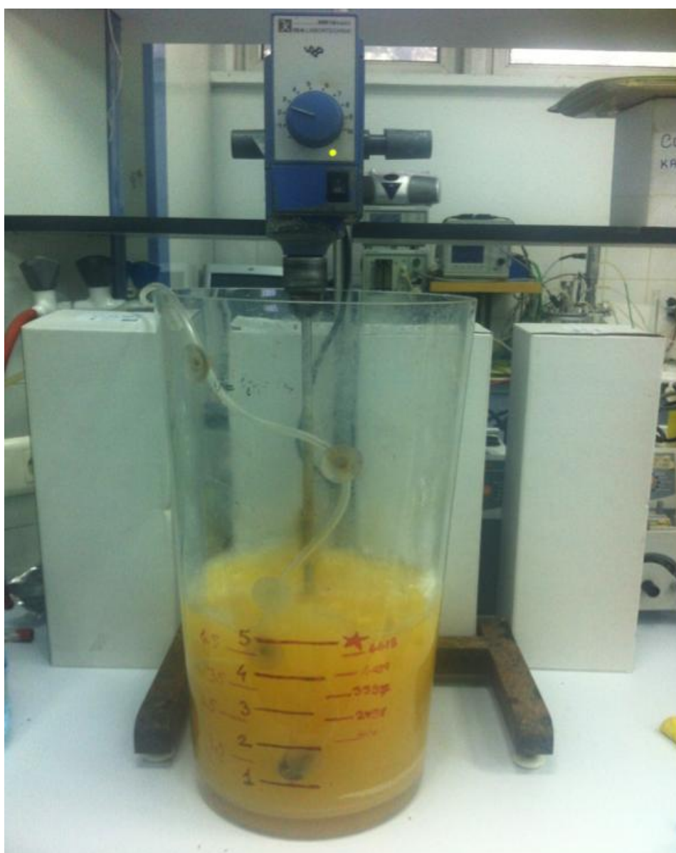
Figure 3.6 : Batch reactor feeding with peptone mixture.
