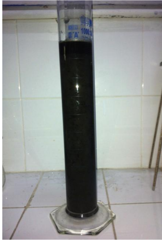
Figure 3.2 : Settled olive mill wastewater after coagulation flocculation.
