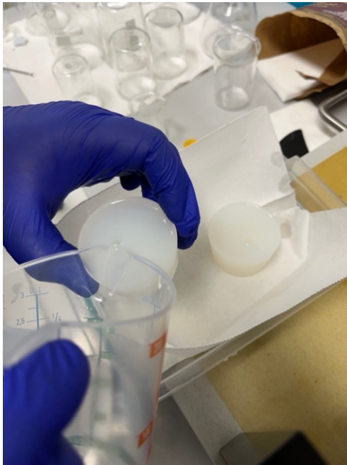
Figure 3.10. Negative Mould Printed with SLA 3D Laser to Mould Designed Lenses
