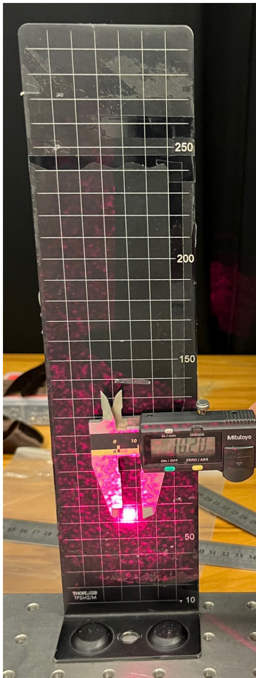
Figure B.2. Measurement of Laser Diameter (Left: 10.2mm, Right: 9.35mm)
