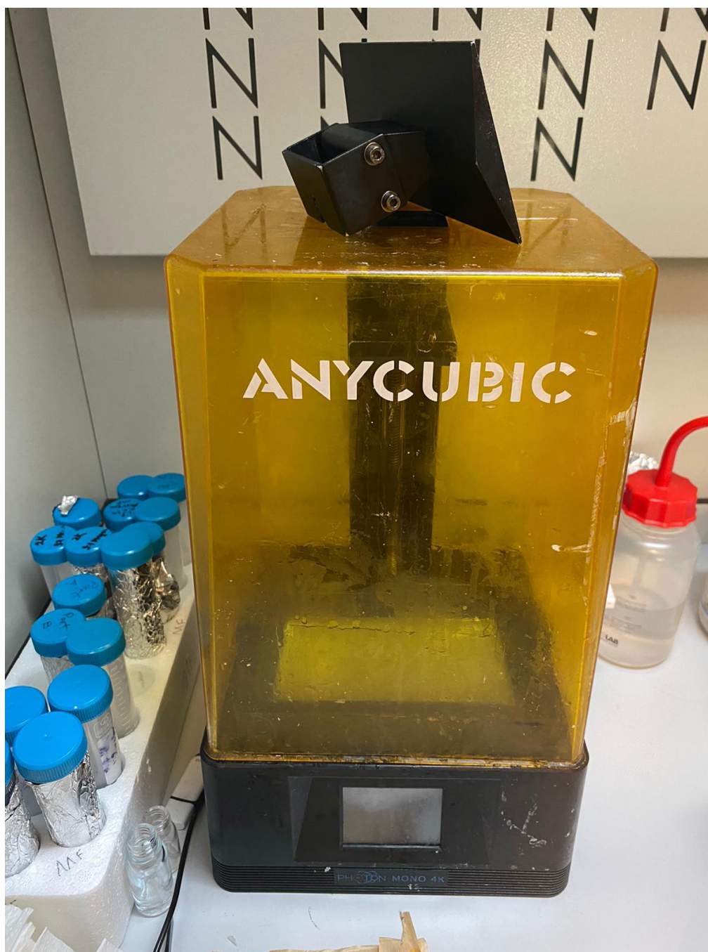
Figure 2.4 Photograph of the Anycubic 3D printer used to manufacture molds used in this experiment.
