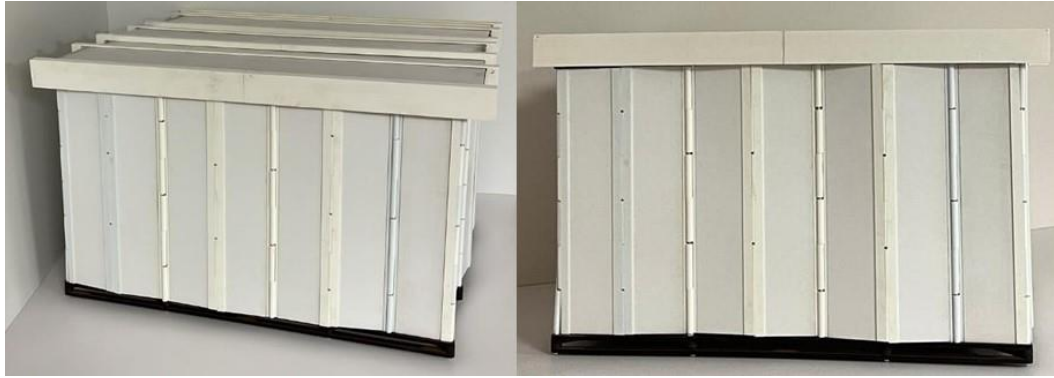
Figure 5.8. Perspective and front view of Shelter Module X physical model in deployed configuration
