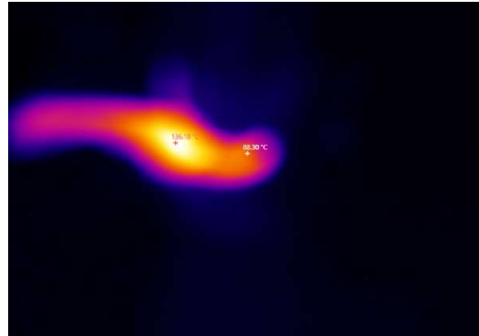
100 mm/dak, 1500dev/dak Deney: 20, Sıcaklık: 136.18°C
