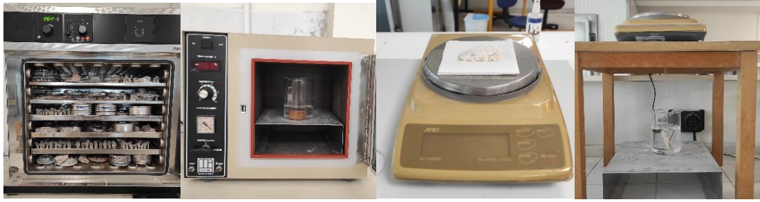
Figure 4. 6. a: Oven for drying samples b: Precision balance used to weigh dry and saturated samples c: Samples in vacuum oven d: Archimedes weight measurement
