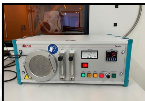
Figure 6.16 Plasma treatment device
