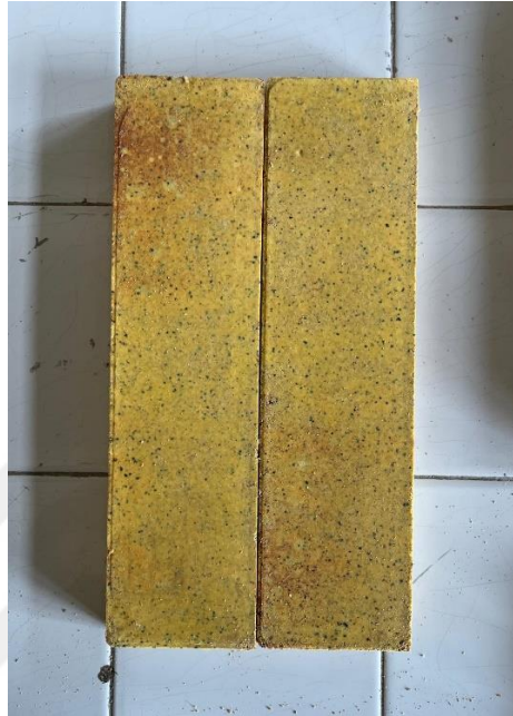
Figure 4.6 Produced Composite Material (30x8x2.5cm)
