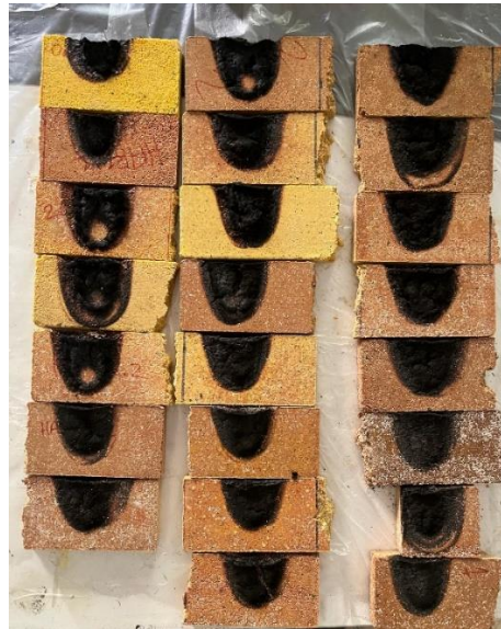
Figure 5.15 Appearance of the samples after 5 minutes of combustion test
