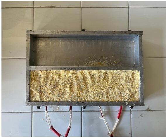
Figure 4.4 Hand Lay-Up Method for Transferring Mixtures into the Mold
