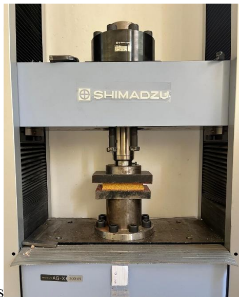
Figure 4.7 Compressive Strength Test
