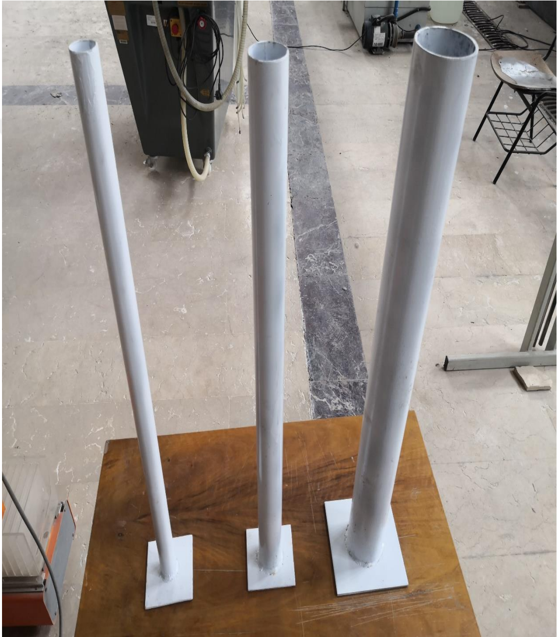
Figure 4.3 The pier models with 3 cm, 5 cm, and 7.5 cm.
