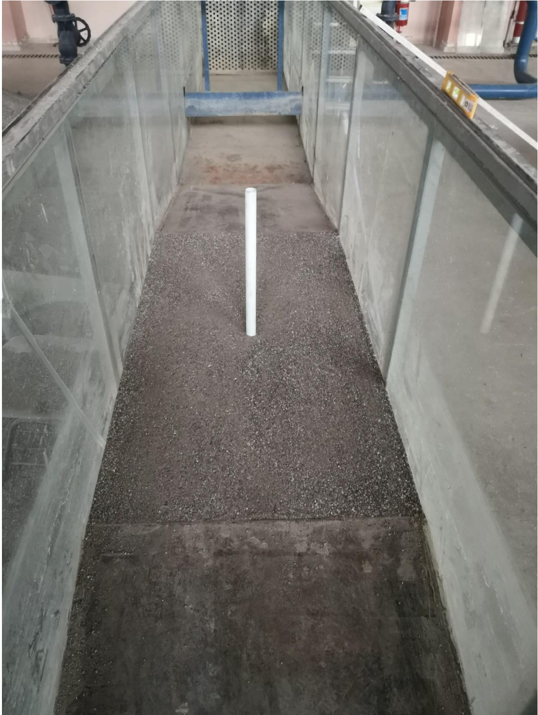
Figure 4.8 Leveled bed and ready for run.
