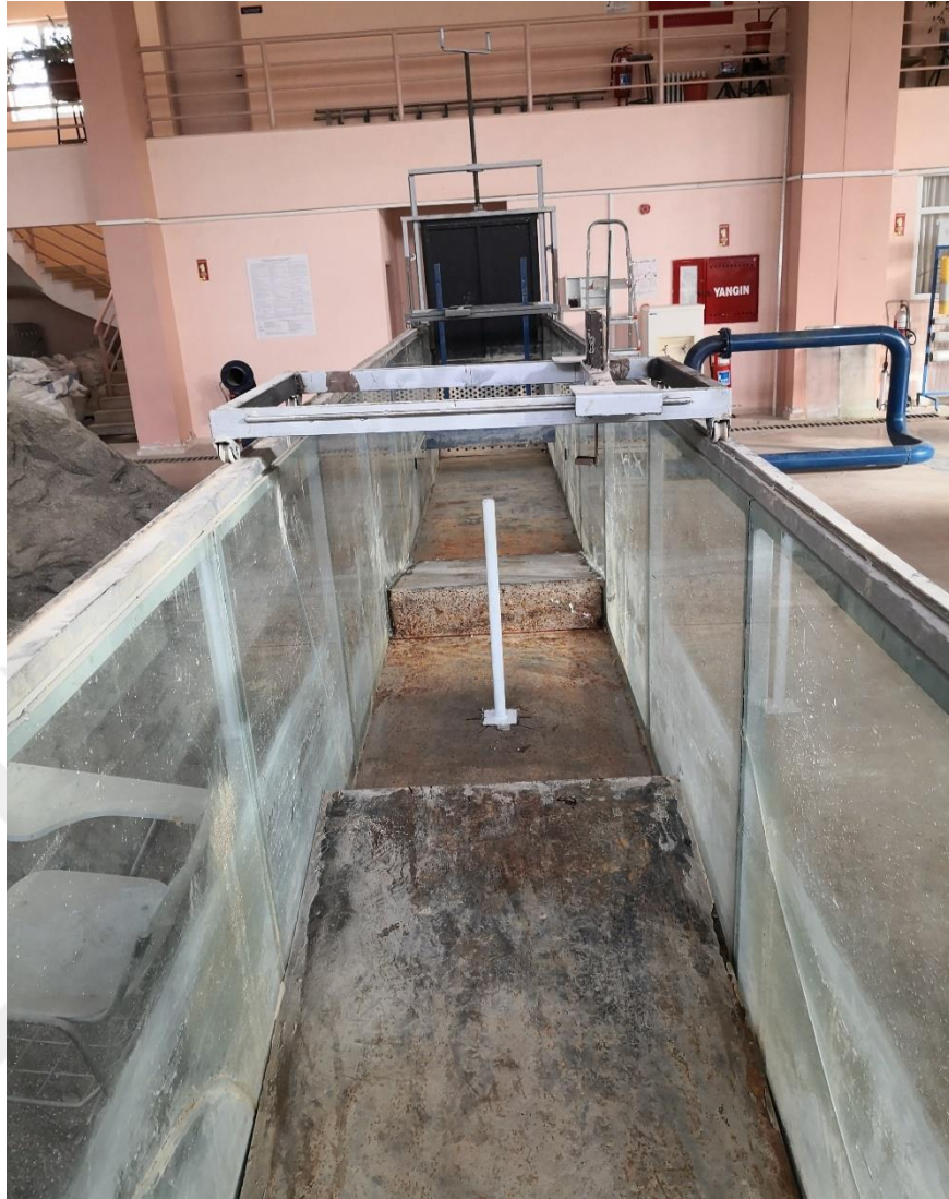
Figure 4.6 Test section and Pier installation.
