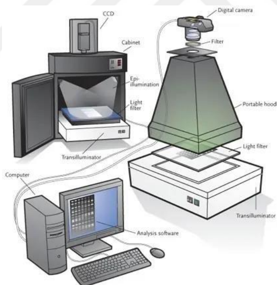
Figure 13: Explanatory Image of Gel Documentation System (SMACgig World,2023)
