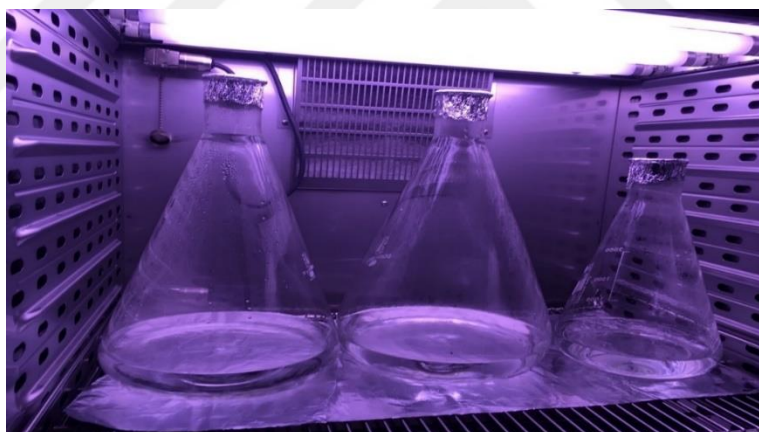
Figure 3.3. Incubation of the inoculum in the test medium done in the temperature-controlled growth chamber under continuous illumination
