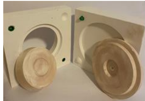
(Model kalıbı, model ve model takozu)
