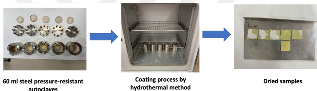
Figure 2.3 Steps of coating Kevlar™ fabrics by the hydrothermal method.
