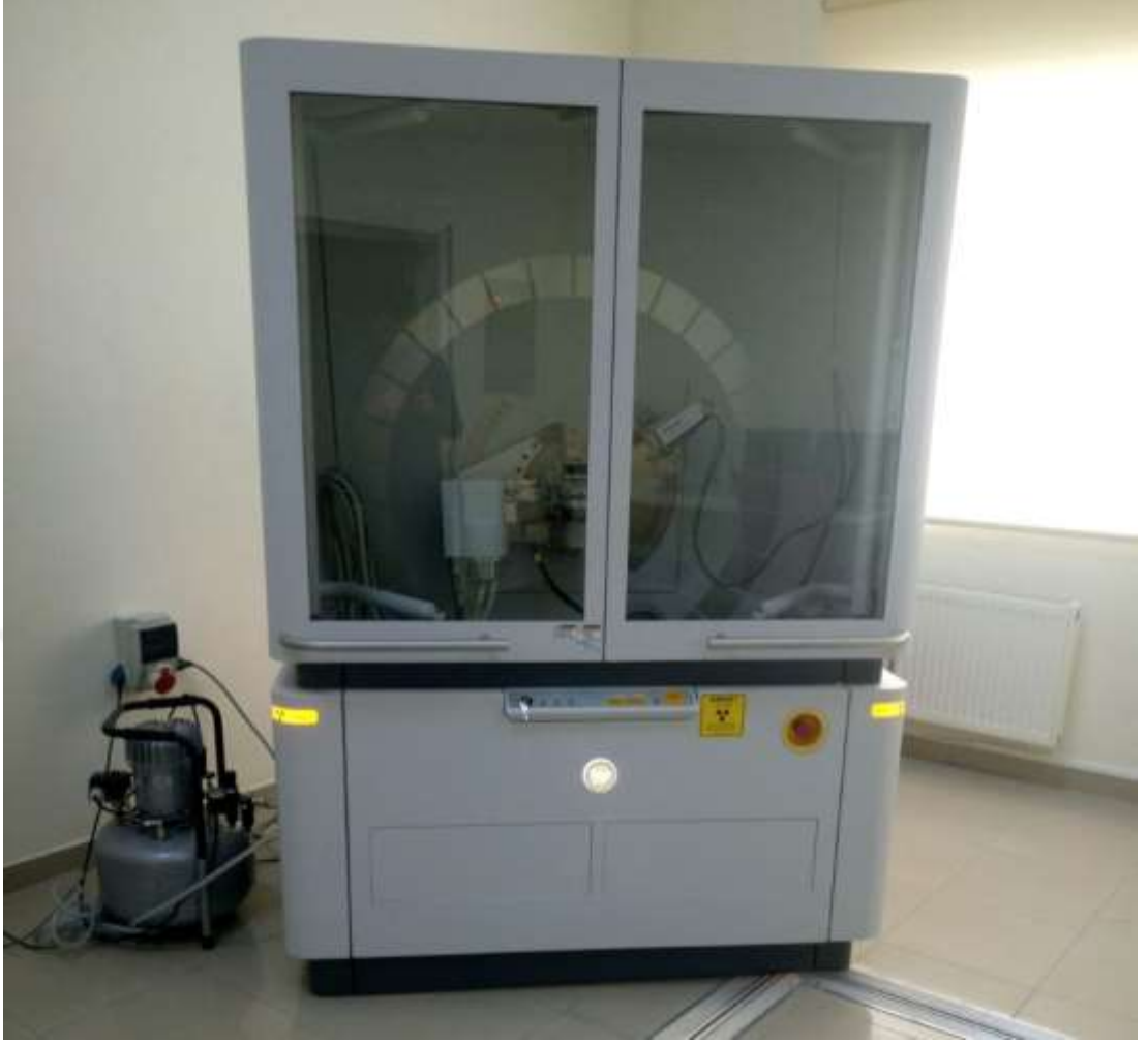
Şekil 2.3. Panalytical marka empyrean model XRD
