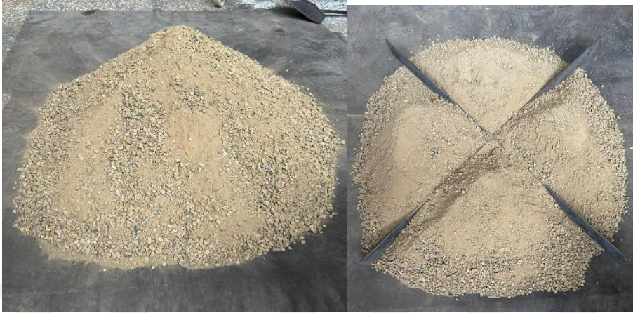
Figure 3.1 Cone and Quartering
