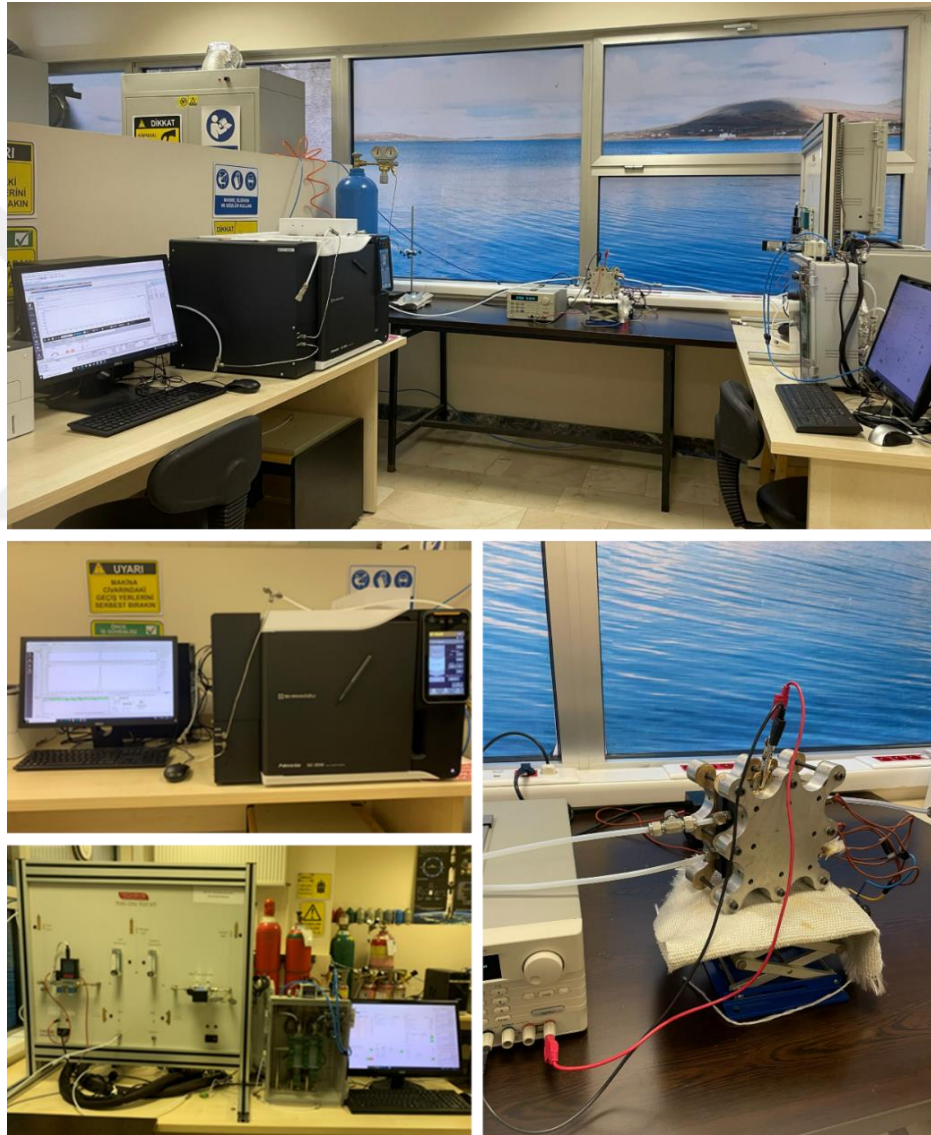
Figure 4.4 Images of the HT-ECHP test station
