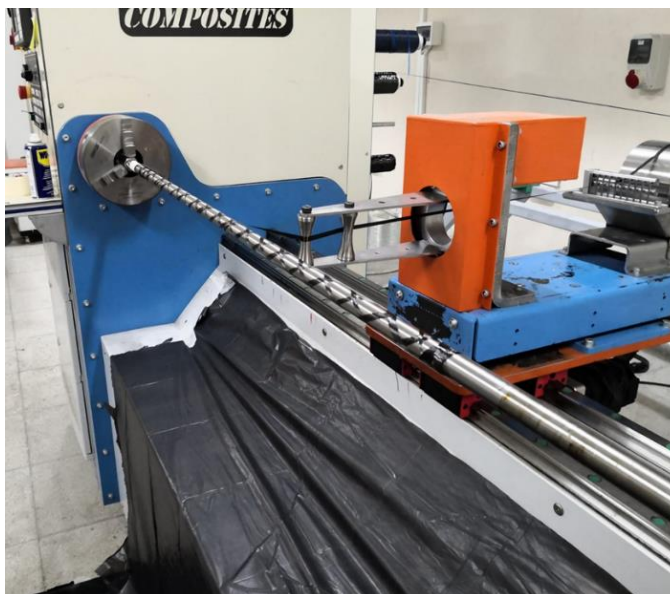
Figure 3.11 Production of [\pm 45]_6 lay-up composite rod
