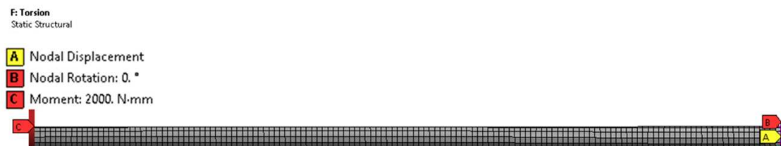
Figure 5.6 Boundary conditions of torsional stiffness model
