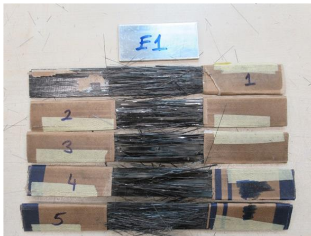
Figure 7.1 0^\circ oriented specimens after tensile test
