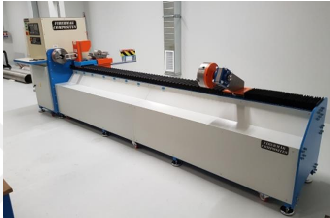
Figure 3.10 General view of 4-axis filament winding machine
