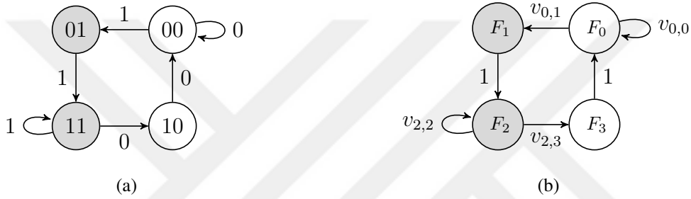
Figure 3.2: (a) An FSTD that represents an SP-LOCO constrained sequence, (b) The same FSTD with transition probabilities on the edges.
