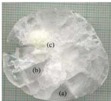
Figure 2.13 The photograph of \text{LiB}_3\text{O}_5 crystal ingot showing (a) transparent (b) translucent and (c) opaque regions. Grid scale: 1mm per division (Sangeeta and Sabharwal 2006).
